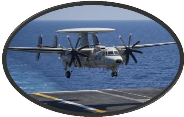
**Northrop Grumman E2-D:** Primary Naval Battle Management / Command & Control aircraft. Vital for aircraft carrier operations. “D” versions in Full Rate Production now to replace all older “C” versions in service. Also operated by 7 foreign militaries – notably Japan to counter China threat.
