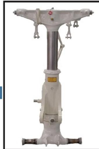
Nose Landing Gear for E2-D Naval Aircraft
